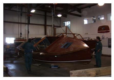
doesn't take much force. Once the boat is off the ground, we start raising the hoist on one side, and then lowering on the other. The friction of the strap on the hull starts rolling it over.
